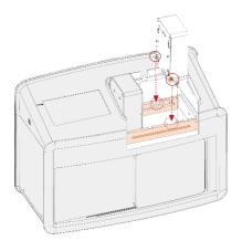
**Step 1** Locate the gearbox under guide rail
